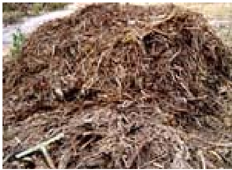
Sugarcane waste bagasse for producing cane coal briquette
