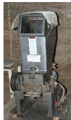
Shredder for kitchen waste
