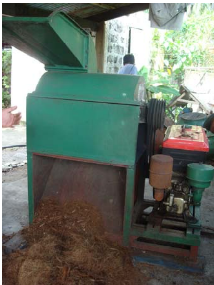
Shredder at MRF station
